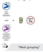
The headsets complete **Mesh Grouping**. The new members will hear a voice prompt as their headsets automatically switch from **Open Mesh** to **Group Mesh**.
