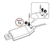
The WiFi Adapter will automatically restart with the three LEDs on.
