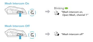
**Note:** When **Mesh Intercom** is on, the **SMART HJC 50B** will automatically connect to nearby **SMART HJC 50B** users and the headset will be in **Open Mesh (default: channel 1) initially**.
