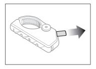
Remove the plastic tape from the battery slot to begin using the Remote Control.
