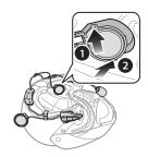
[Make sure that the Microphone wire is not pressured by the speaker unit when installed]
