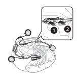
4. Insert longer hook of the right speaker unit into bottom hole of the speaker pocket. Place the Microphone wire under the bottom hook of the speaker unit when installing. Insert shorter hook of the right speaker unit into the top hole of the speaker pocket.
