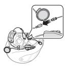
2. Tighten the two long screws until the Bluetooth module is fastened firmly to the helmet.
