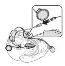
2. Tighten the two long screws until the Bluetooth module is fastened firmly to the helmet.
