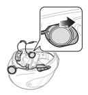
[Once installed, the position of the speaker unit can be adjusted to rider's ear position]
