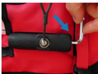
G. Finish tightening the cap with the 5mm allen wrench. The end cap must be tightened until no thread is showing and the cap will turn no more.
