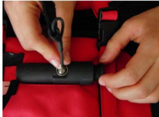
F. While ensuring that the ball bearing remains flat in its set, begin to tighten the cap manually.
