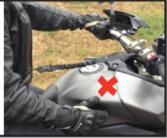
The fixing point resists over 150kg. For example, do not use a plastic part.
