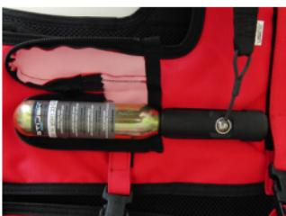
H. Now insert your new CO2 cartridge ensuring that it is screwed fully by hand so that thread doesn't shows. Don't not over tighten. The cartridge must be practically in contact with the plastic of the trigger. If not tight enough and the cartridge will not be fully pierced, inducing slow or no inflation.
