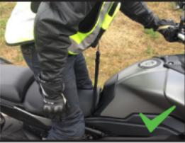
Do not attach the strap to the handle bar
