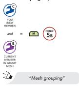
The headsets complete **Mesh Grouping**. The new members will hear a voice prompt as their headsets automatically switch from **Open Mesh** to **Group Mesh**.
