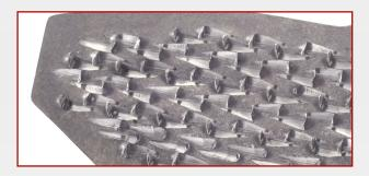
4. The pad material of the CRQ pads contains carbon, which makes it very sensitive and means it requires careful handling when not installed. Corners can quickly lift up if the pads fall onto the floor or bump into sharp edges.
