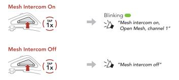
Note: When Mesh Intercom is on, the SRL-Mesh will automatically connect to nearby SRL-Mesh users and the headset will be in Open Mesh (default: channel 1) initially.
