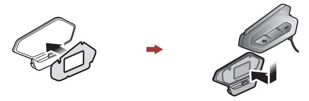
3. Insert the back plate of the clamp between the internal padding and external shell on the left side of the helmet.
