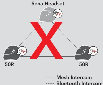
If Bluetooth intercom is accidentally turned on during Mesh Intercom communication between 50R headsets, as shown below, you will hear a voice prompt, "Mesh intercom disabled, Bluetooth intercom connected" every 1 minute. If you turn off the Bluetooth Intercom or turn off the Mesh Intercom, the voice prompt will no longer come out.
