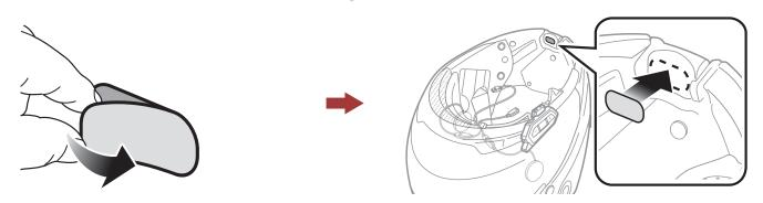
2. Attach the wired microphone to the hook and loop fastener for wired microphone.
