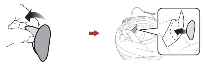
2. Attach the speakers to the hook and loop fasteners for speakers inside the helmet.
