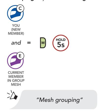
2. The headsets complete **Mesh Grouping**. The new members will hear a voice prompt as their headsets automatically switch from Open Mesh to Group Mesh.
