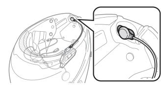
3. Align the arrows on the main unit and microphone cables and insert the microphone cable into the microphone connector.
