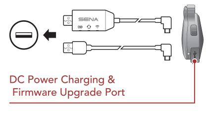
You can charge the headset by connecting the **WiFi Adapter** or a **USB Power & Data Cable (USB-C)**.
