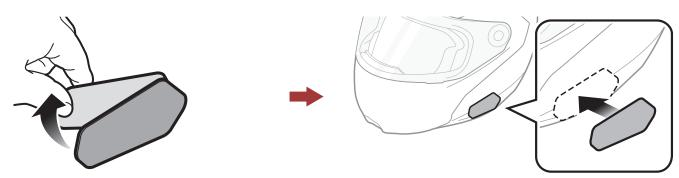
3. Peel off the cover of the adhesive tape of the hook fastener for main unit and attach it to the back plate of the main unit.
