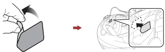
2. Attach the wired boom microphone's mounting plate to the hook and loop fastener.
