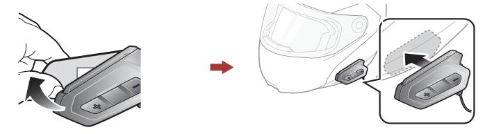
4. Make sure that the main unit sticks on the helmet firmly. Maximum adhesion occurs after 24 hours.
