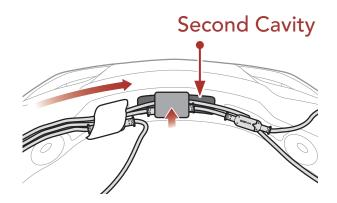
**Note:** Do not cover the snap fastener with the aligned cables. Make sure the aligned cables are placed above the snap fastener.
