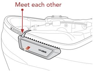
**Note:** Make sure that the main unit is firmly attached to the helmet. Maximum adhesion occurs after 24 hours.
