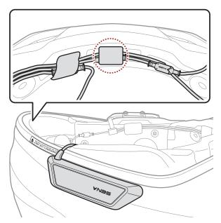
2. Remove the battery cable from the battery connector and then insert it back in.
