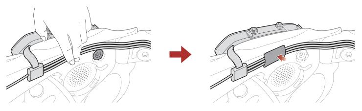
**Note:** Do not cover the snap fastener with the aligned cables. Make sure the aligned cables are placed above the snap fastener.
