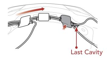
**Note:** Do not cover the snap fastener with the aligned cables. Make sure the aligned cables are placed above the snap fastener.
