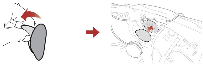
14. Attach the **speaker (R)** and the speaker pad to the hook and loop fastener use for the speaker inside the helmet.
