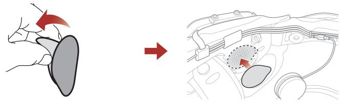
6. Attach the **speaker (L)** and the speaker pad to the hook and loop fastener use for the speaker inside the helmet.
