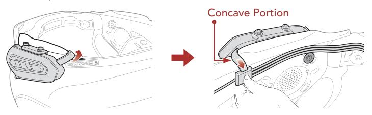
2. Secure the cables with adhesive tape while aligning them.
