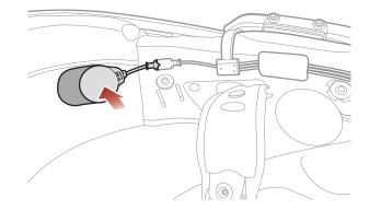
**Note:** Do not cover the snap fastener with the microphone cable. Make sure the cable is placed above the snap fastener.
