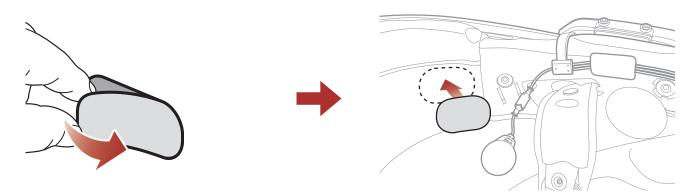
4. Attach the wired microphone to the hook and loop fastener for wired
