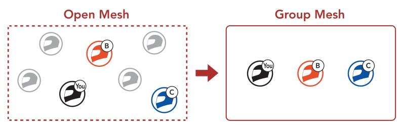
To enter Mesh Grouping to create a Group Mesh, press and hold the Mesh Intercom Button for 5 seconds on the headset of the users (You, B, and C).
