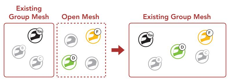
To enter Mesh Grouping to join the Existing Group Mesh, press and hold the Mesh Intercom Button for 5 seconds on the headsets of one (You) of the current users in the Existing Group Mesh and the new users (D and F) in Open Mesh.
