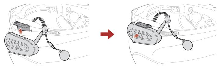
**Note:** Make sure that the main unit is firmly attached to the helmet. Maximum adhesion occurs after 24 hours.
