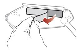
5. Attach the main unit to the clamp, and attach the back of the main unit to the left side of the helmet with double-sided adhesive tape.
