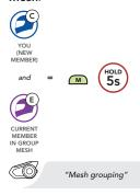
The headsets complete **Mesh Grouping**. The new members will hear a voice prompt as their headsets automatically switch from **Open Mesh** to **Group Mesh**.
